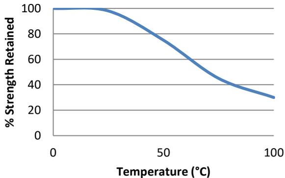
Fully cured lap shear specimens conditioned to pull temperature for 30 minutes before testing at temperature.
