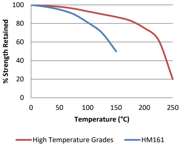
*"Hot strength" Breakaway strength on M10 Zinc plated bolts according to ISO 10964. Cured at 23°C for 24 hours then conditioned for 30 minutes at testing temperature.*
