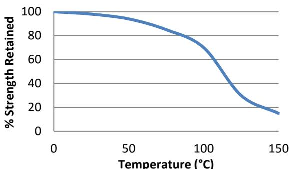
"Hot strength" shear strength tests performed on mild steel. Fully cured specimens conditioned to pull temperature for 30 minutes before testing at temperature.
