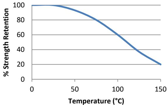
"Hot strength" shear strength tests performed on mild steel. Fully cured specimens conditioned to pull temperature for 30 minutes before testing at temperature.
