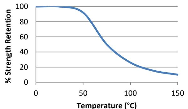
"Hot strength" shear strength tests performed on mild steel. Fully cured specimens conditioned to pull temperature for 30 minutes before testing at temperature. ET5364 can withstand higher temperatures for brief periods (such as for paint baking and wave soldering processes) providing the joint is not unduly stressed. The minimum temperature the cured adhesive can be exposed to is -40°C (-40°F) depending on the materials being bonded.
