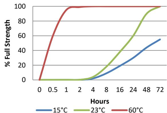
Graph shows typical strength development of bonded components. An increase of 8°C in temperature will halve the cure time. Lower temperatures will result in a slower cure time.
